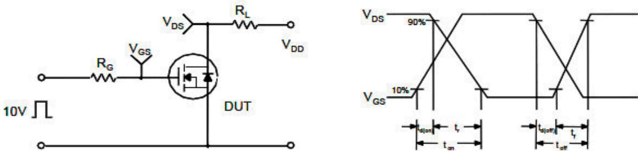
Unclamped Inductive Switching Test Circuit & Waveforms
