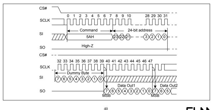
Figure36. Read Serial Flash Discoverable Parameter command Sequence Diagram
