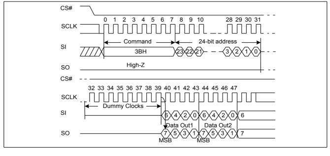
Figure10. Dual Output Fast Read Sequence Diagram
