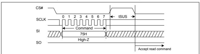
Figure29. Program/Erase Suspend Sequence Diagram
