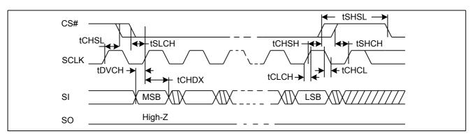
Figure41. Output Timing
