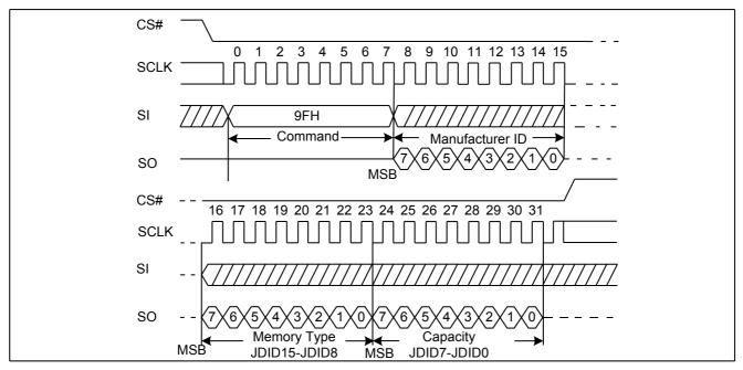
Figure28. Read Identification ID Sequence Diagram
