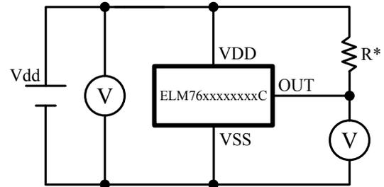
\* Pull up circuit is necessary for N-ch output only.
