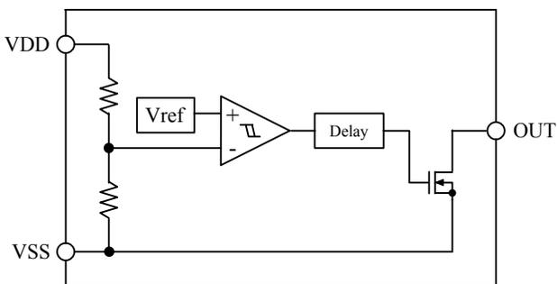
N-ch open-drain output for RESET output logic
