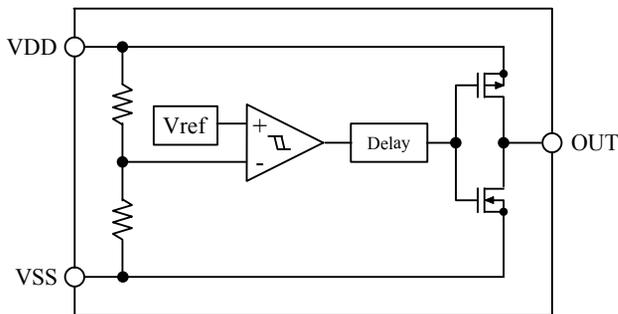
CMOS output for RESET output logic
