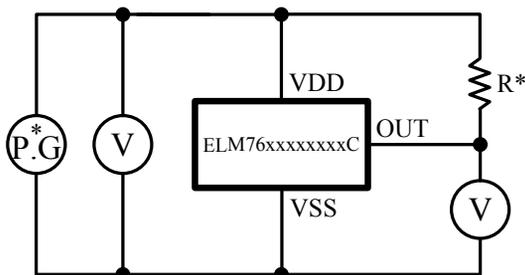
\* Pull up circuit is necessary for N-ch output only.
