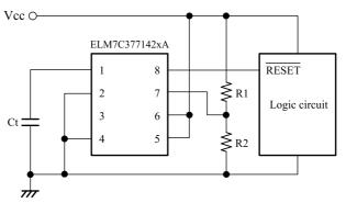
The Vsa detection voltage can be adjusted externally.
