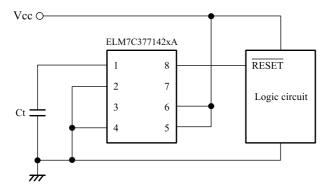
2) 5V Power Supply Voltage Monitor (Externally Fine-Tuned Type)
