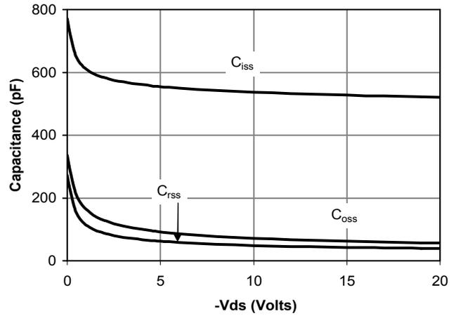
Figure 8: Capacitance Characteristics
