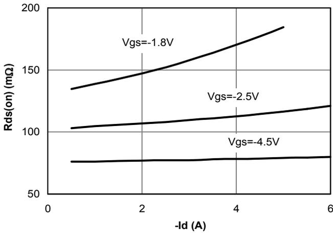
Figure 3: On-Resistance vs. Drain Current and Gate Voltage
