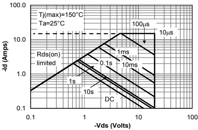
Figure 9: Maximum Forward Biased Safe Operating Area (Note 5)
