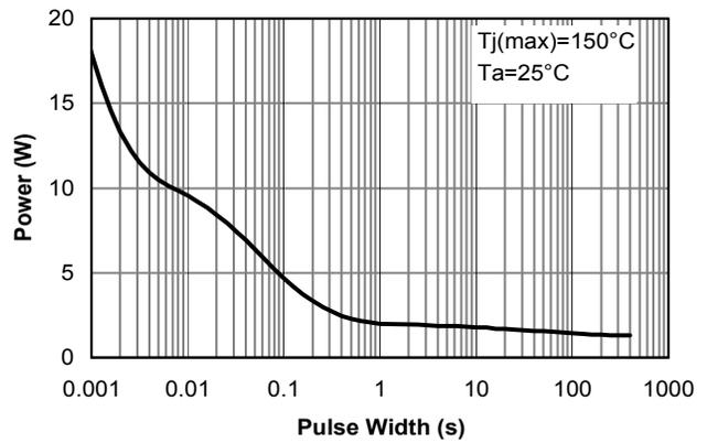
Figure 10: Single Pulse Power Rating Junction-to-Ambient (Note 5)
