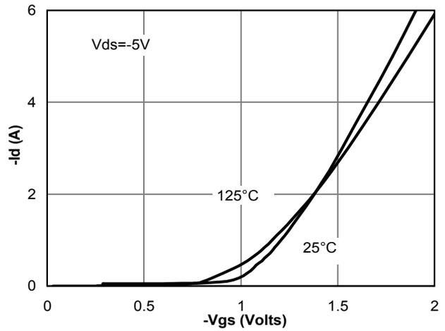
Figure 2: Transfer Characteristics
