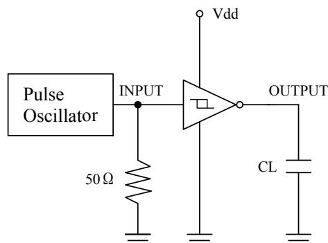
\* Output should be opened when measuring current consumption.
